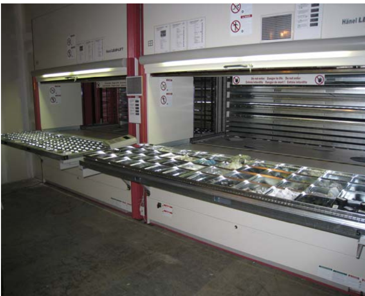
Two Hänel Lean Lifts eliminated over 80 shelving units and eliminated the need for an entire steel deck mezzanine
