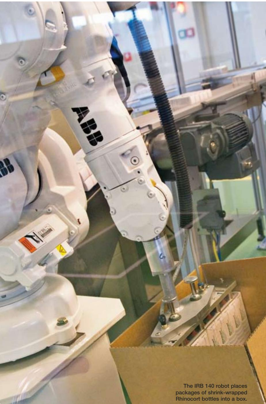
The IRB 140 robot places packages of shrink-wrapped Rhinocort bottles into a box.
