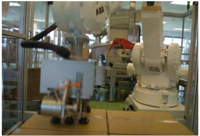
The second and bigger ABB IRB 4400 robot in the FlexCell has several functions. First, it erects the cardboard boxes for its little brother. Once these are filled, it reaches over and lifts them, also with suction pads, up to an inkjet printer that writes directly on the cardboard the product information, batch number and a barcode. At the same time, a barcode reader checks the barcode. Then the robot palletizes the boxes in one of two pallet areas.
