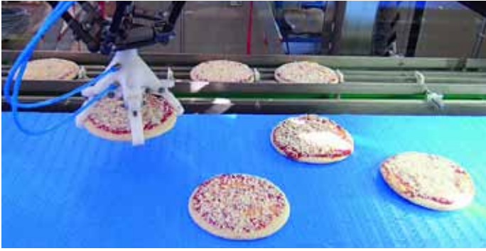
Picking pizzas from a moving conveyor belt. One wrong move and all the accoutrements are spilled onto the factory floor.
